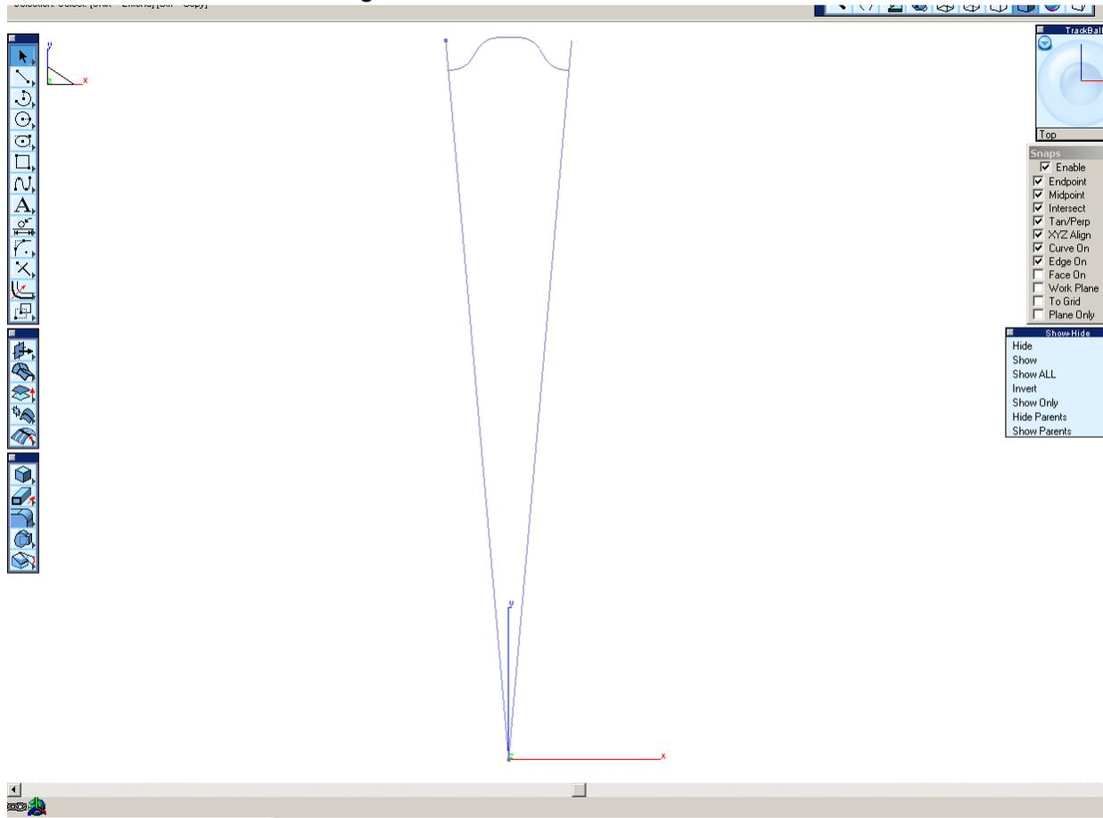
After finishing the tooth, create the solid gear.
