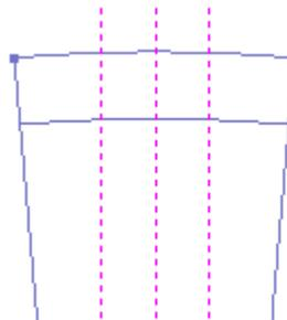
*Create one parallel line off of the original. The rest of the lines can be created by entering different + & - offset values into the Status Line data box.*
