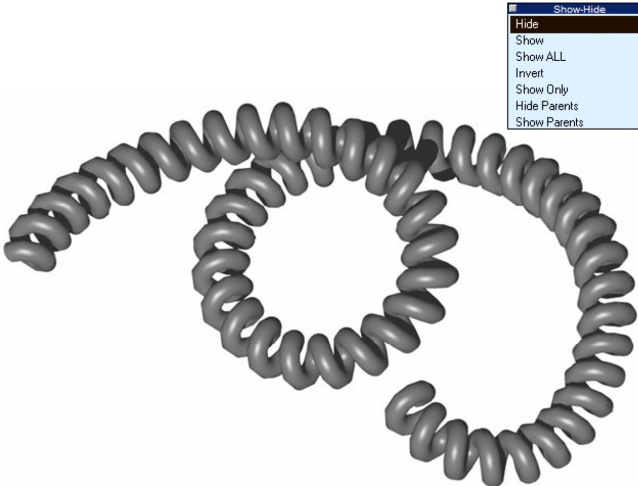
10. It is also possible to explode more than one edge of the twisted rectangle shape. These edges can be used to create double helix or braided shapes.
