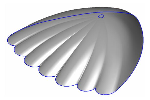
Using the **Skin Surface** tool, create a surface by holding the Shift key and selecting all three objects, the profile, the circle and the point. This will create a nice shape except that the leading edges are sharper than they should be. The next step shows how to quickly round the perimeter.
