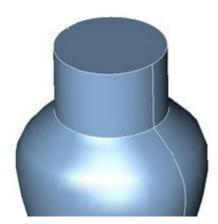
11. Blend the bottom edge with a nice, large radius.
