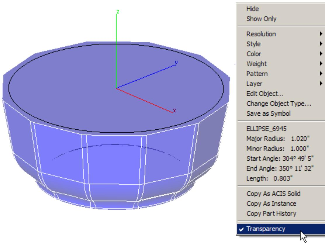
17. Select the **Extrude** tool with the **Distance** option, extrude the circle about - **1.75"** and give it the same amount of draft as the outer shape (**-10** degrees).
