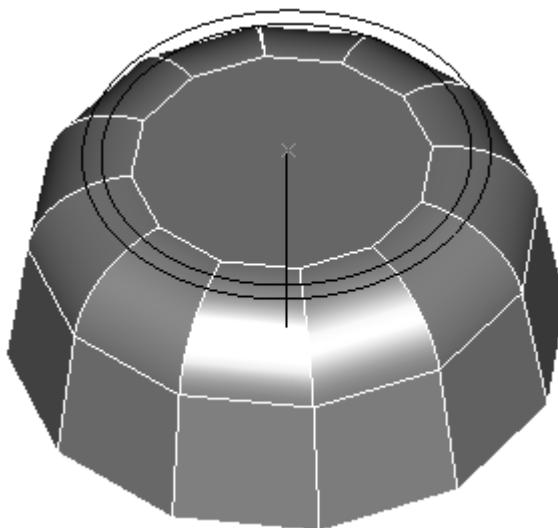
9. Select the **Extrude** tool and specify **Vector** option in the Message Line. Extrude the two circles downward some distance so that they protrude into the bowl. Hold the SHIFT key and select both circles at the same time. Release SHIFT and specify the vector of extrusion in an empty space along the z axis.
