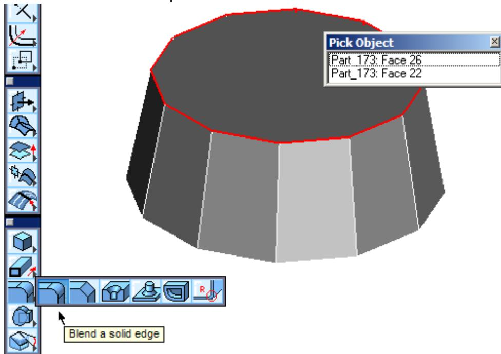
6. Below is the resulting shape. To make edges look like the picture below, use **View>Shade Options** to display the window and edit the parameters of the edges displayed. Set the Static Shade option to *Phong w/Edges* then click OK.
