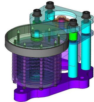
Gleeson designed this fluid-dampened servo mechanism for a camera crane with a clutch pack that applies torque without requiring a large gear train.
