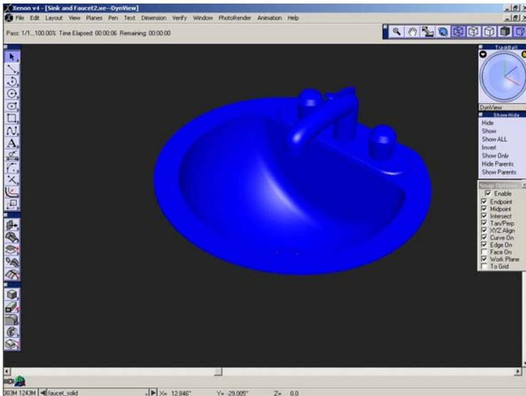
The part that we are going to be most interested in right now are the knobs. To get a better view of them you can go to the front view of the drawing by selecting **Front View** from the drop-down list at the bottom of the Trackball.
