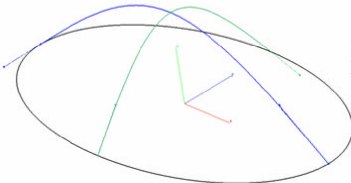
Draw a second spline over the top, perpendicular to your first spline.
