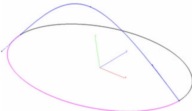
Draw a spline with 3 points that connects to the endpoints of the ellipse halves.
