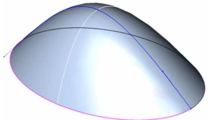
Use the Skin Surface tool and select all three curves by using the Shift key. A surface like this should be created.
