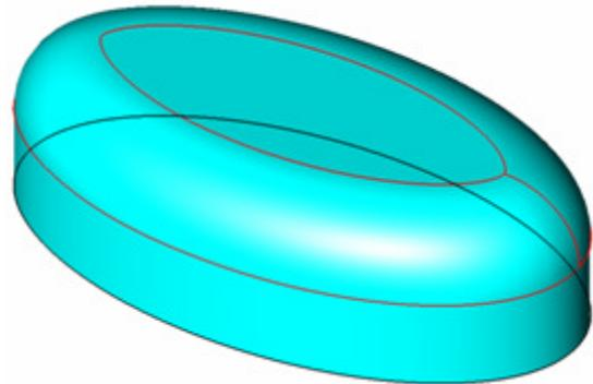
Use the Blend tool to round off the edge of an extruded shape. This is easy, but it the shape is limited by the capabilities of the Blend tool.
