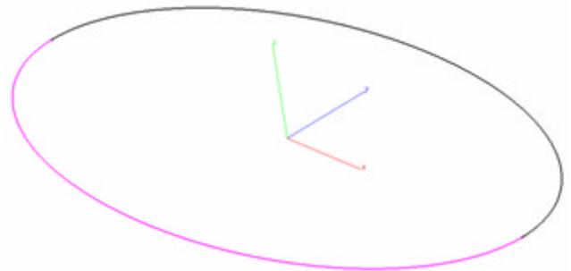
Use the **Divide Curve** tool to split the ellipse into two.
