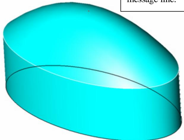
First select the face to dome and then define the direction/height for the dome.
