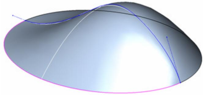
By making your domed shape using a surface that is defined by a spline, you have the ability to adjust the control vertices thereby changing the shape of the surface.
