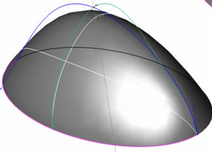
Because the net surface is defined by several splines, it offers more control over the shape of the surface
