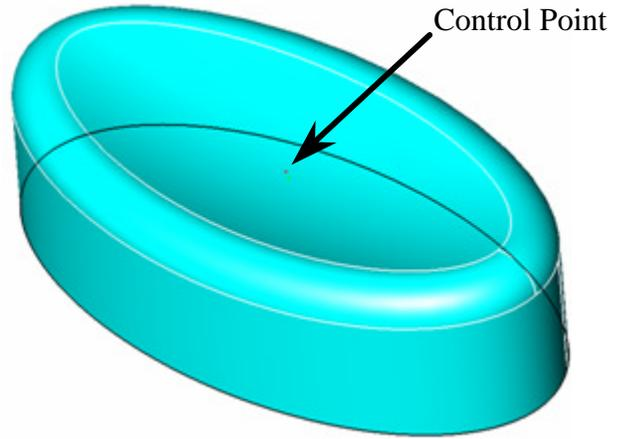
You can also create a concave dome shape by pulling the control point downward (align z).
