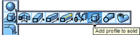
12. Extrude the sketch to form a solid by selecting the base extrusion solid, then the sketch profile and finally the two points in the z axis. With the extrusion still highlighted type 40mm in the status line distance field and press the ENTER (Windows) or RETURN (Macintosh) key.
