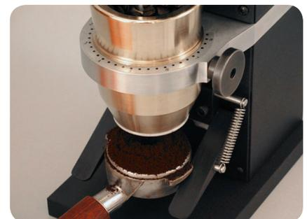
The dosing hopper (top) and the portafilter holder (bottom) are two accessories designed by John for his original espresso grinder, also designed in Xenon (centre) CAD and 3D modelling software.
